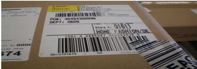
Figure 9 F : Improper label placement. UCC128 label must not be covered by any other labels or tapes
