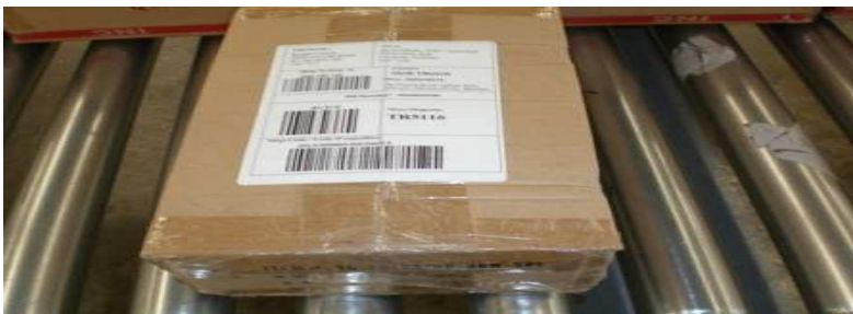
Figure 9 C : Improper label placement. 20 digit SSCC barcode over the carton seams
