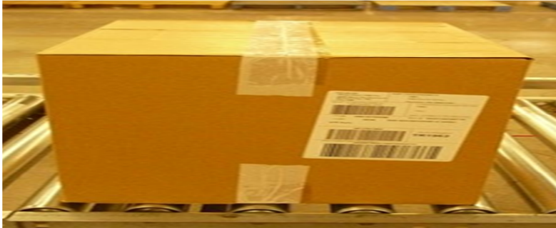
Figure 9 B : Proper label placement. UCC128 label applied to largest flat surface
